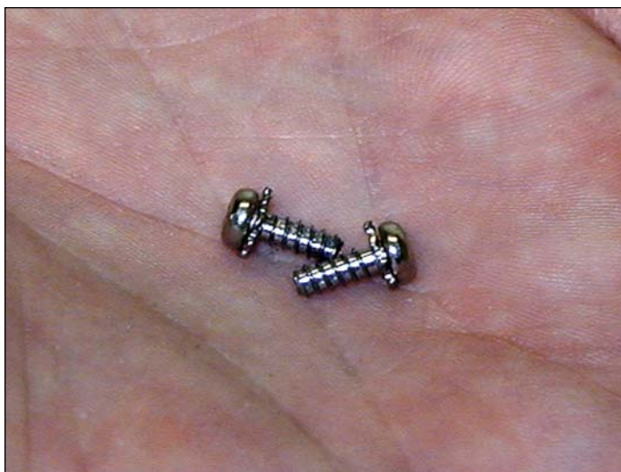
13. On the toner supply chamber right side, Remove the two screws and end cap. Note that these screws have lock washers.
