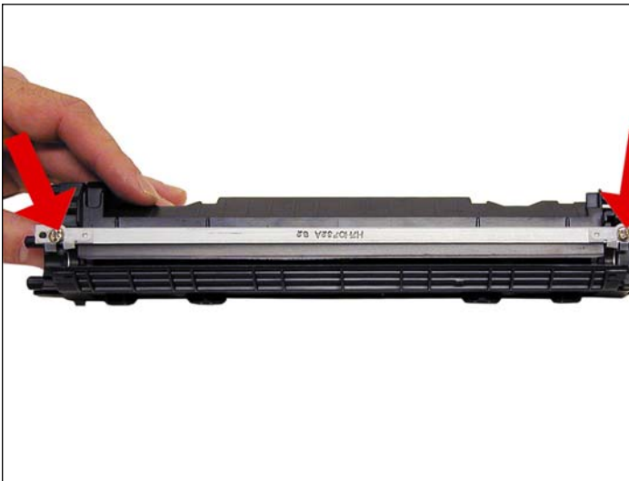
17. Remove the doctor blade and two screws.
