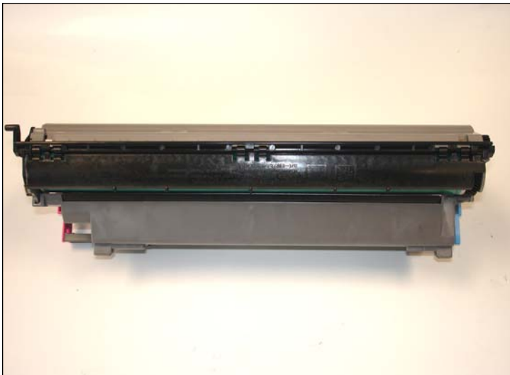
3. Back view of the drum unit.
