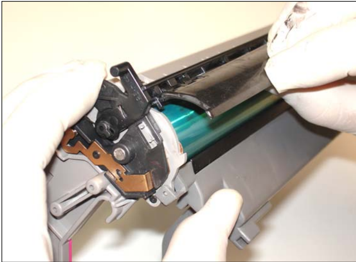
7. Release the drum shutter from the hopper.
