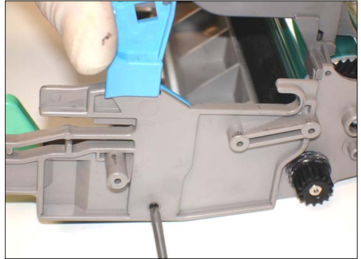
10. Note there are two screws on each side of the cartridge.
