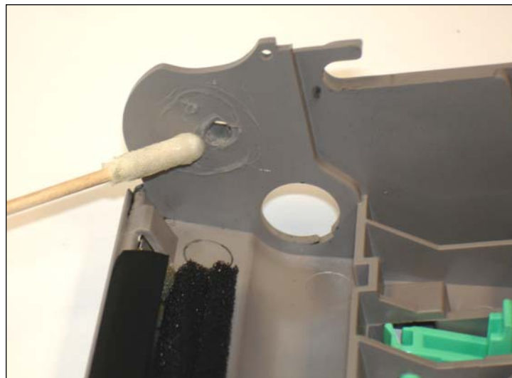
20. Lubricate the drum gear housing with gear grease.
