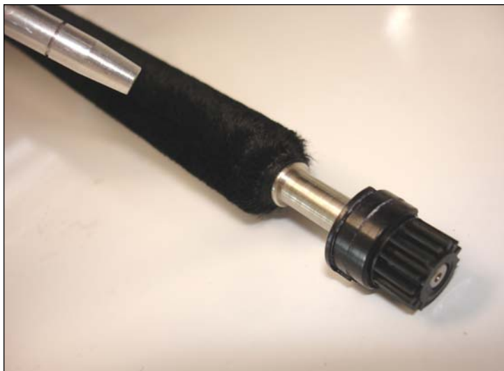
19. Clean the PCR brush with air compressed.
