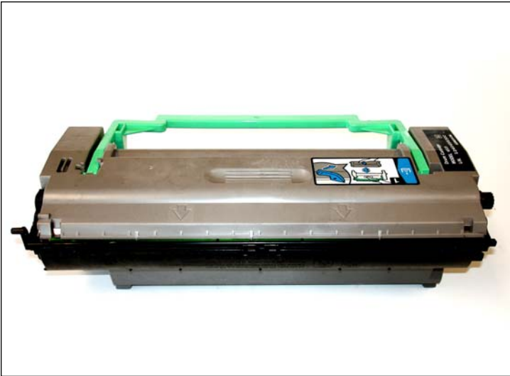
31. Drum unit ready to be used.
