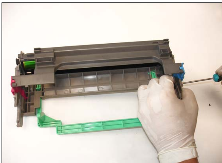
27. Reassemble the fixing arm and place all the screws on each extreme of the drum unit.
