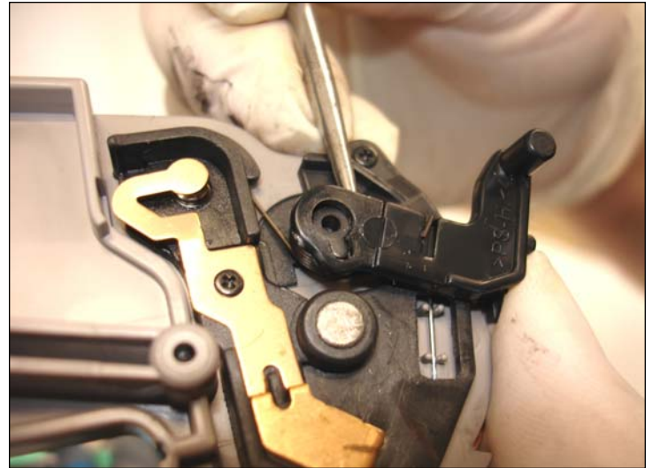
8. Remove the shutter arm from the plastic pin with a small flat-head screw driver.
