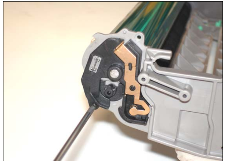
12. Remove the two small black screws from the drum contact plate.
