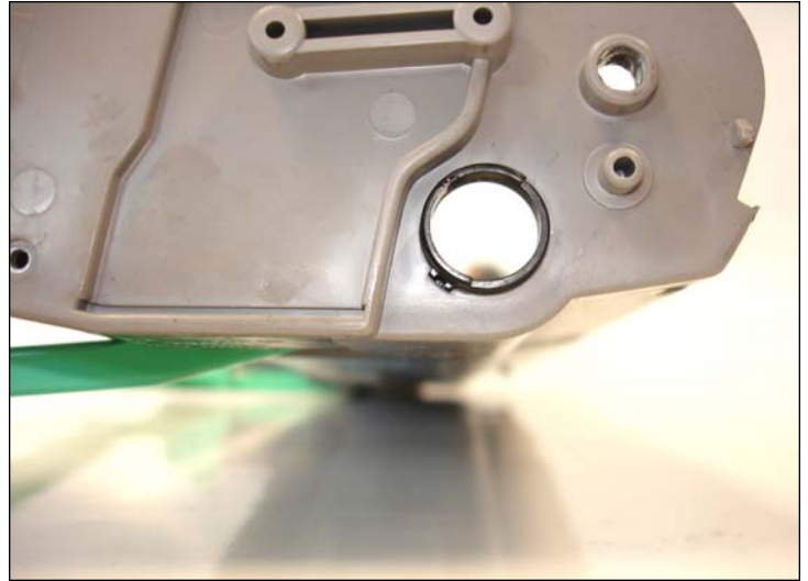
22. Notice the detail of the black PCR bearing. Do not lose it.
