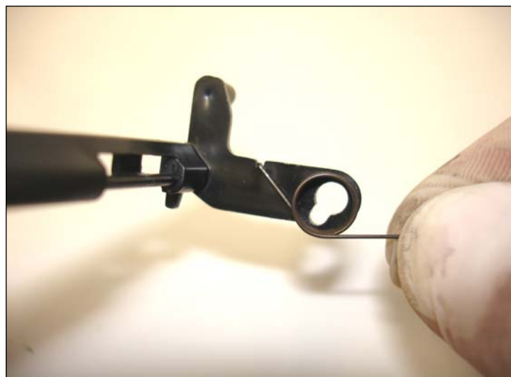
28. Place the spring as shown in the drum shutter arm.
