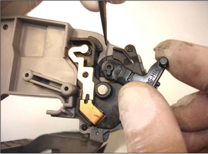
29. Place it in the main cartridge unit using a spring tool or a little flathead screwdriver.
