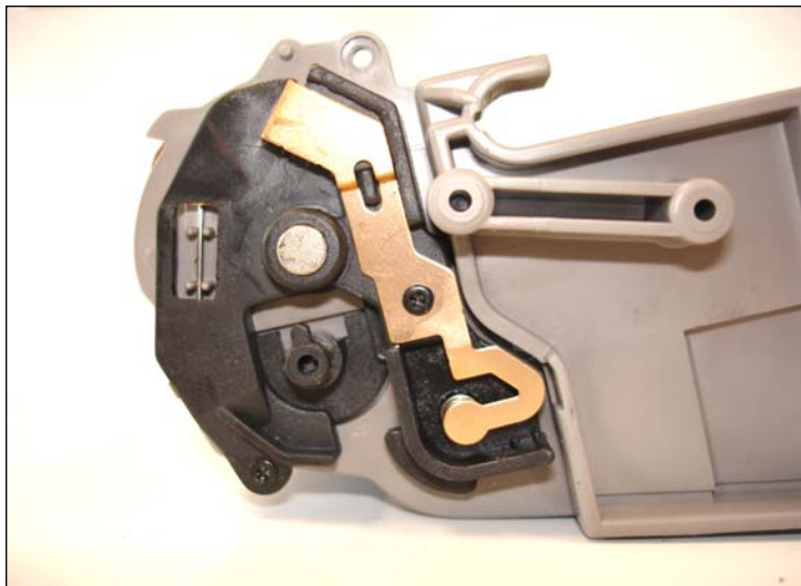
25. Use a Phillips screwdriver to place both small black screws onto the contact end plate.
