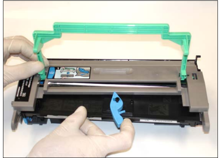
2. Pull the blue plastic handle to free the toner unit.
